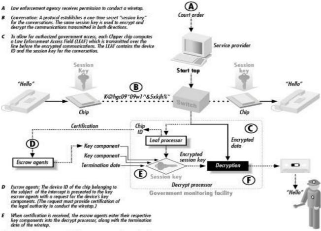
F Inside the decrypt processor, the key components are decrypted and combined to form the device-unique key. Once the decrypt processor has that key, it can decrypt the session key in the LEAF, and then ase the session key to decrypt the communications in both directions.
